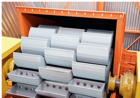
Detail of the elevator axis and buckets.
